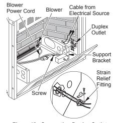
Figure 15 - Connecting Duplex Outlet
